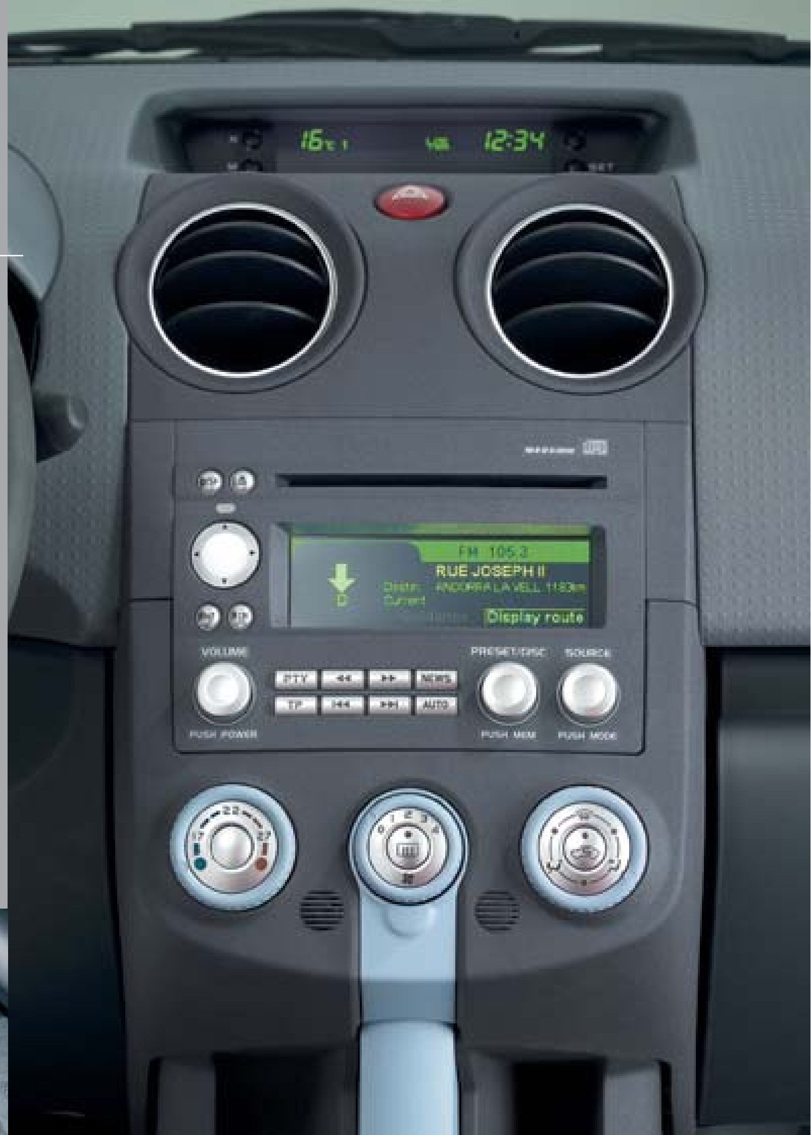
Arrow type navigation system PZ-5000 Colour arrow type navigation system, 4.9" colour display, RDS (EON/PTY) tuner, CD player, CD changer control, telephone mute preparation, trip computer mode switch, 4 x 25W. CD music play is possible while navigation is in use thanks to the internal memory with corridor function. A security code card is supplied with PZ-5000. MZ312960
