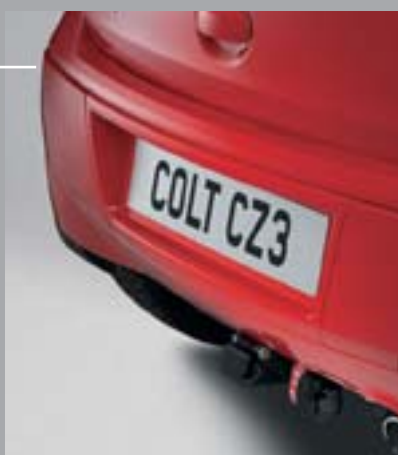
Towbar, detachable With integrated lock. MZ313402
